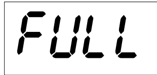
Figure 5. Drive is running at full speed
