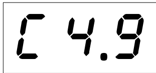
Figure 8. When flashing, the pump is working on Time Dispense Setup Mode ,
